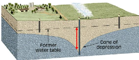
$$\text{水位降下量} = (\text{静水位}) - (\text{動水位})$$
